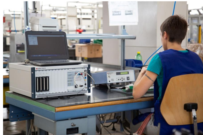
Test of connection of components, insulation, electrical resistance, functional of switches and push-buttons, functional of relays and components with RLC meter
