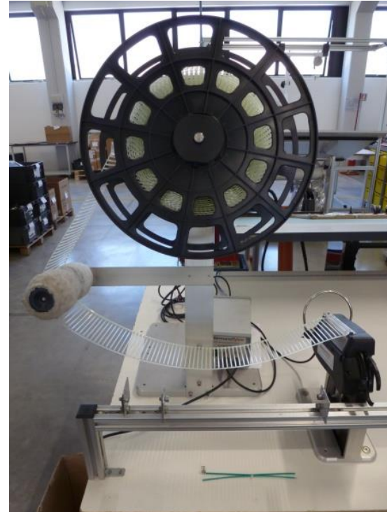
Automatic binding system with cable ties
